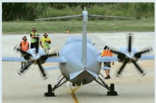
The design of the P.1HH-XP HammerHead aims at being a unique ISR platform, able to climb up to 45,000 feet, loitering quietly at low speed (135 KTAS) for an endurance of up to 15 flight hours and dashing at very high speed (up to 395 KTAS) to target.
