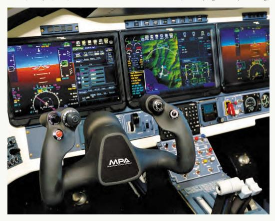
dedicated control panels and monitors to maximize flexibility and crew task allocations while having a direct integration into the aircraft avionics for best mission management and integration of pilot and operators activity.
