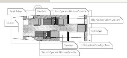
The large, stand up cabin allows installation of a wide range of mission-consoles for flexible operation and special missions work; thanks to the rearward pusher propeller configuration the cabin has the lowest internal noise and vibration level of this aircraft category. The Crew are comfortably located in a stand up operative area with two consoles, one rest seat, a galley and a stand up toilet. With a differential pressure of just 9 psi the cabin has a very low equivalent
